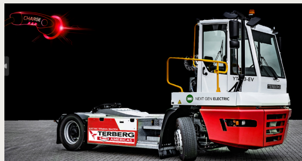
Fully electric yard/terminal tractor
