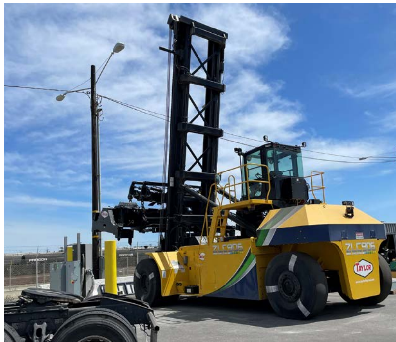
Figure 2 Battery-Electric Top Handler at the Port of Oakland
