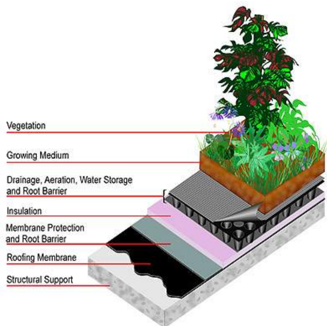
Figure E-3. Green Roof Schematic
