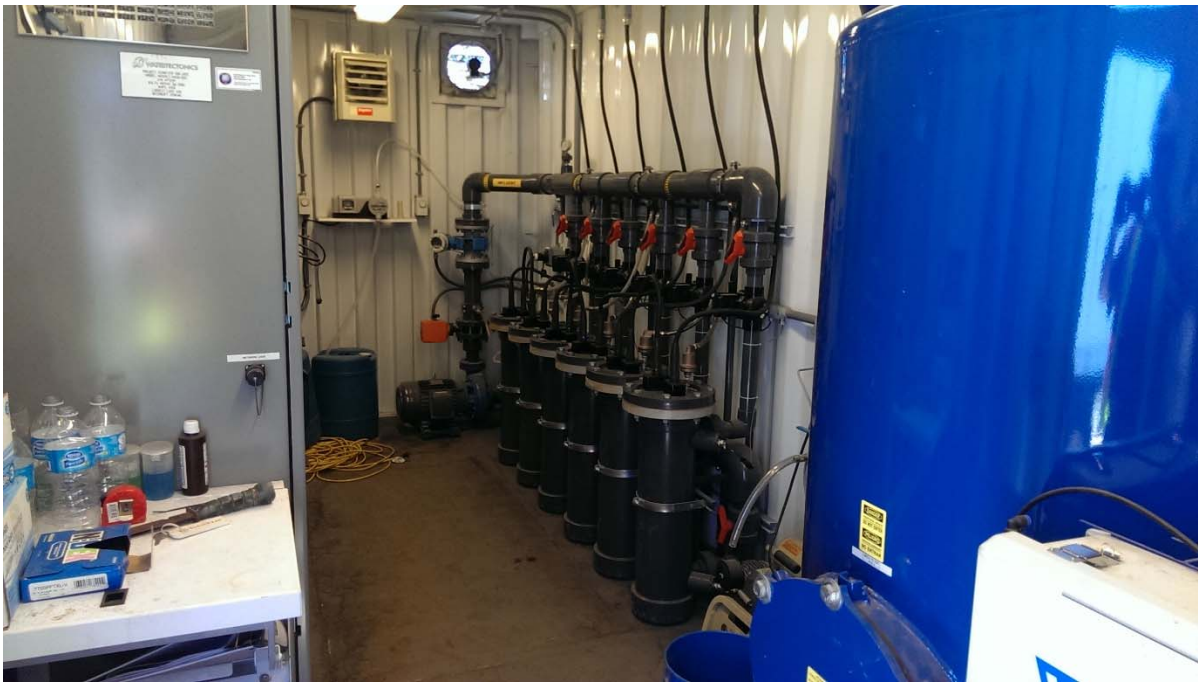
Electrocoagulation (Treatment Cells and Media Filter)
