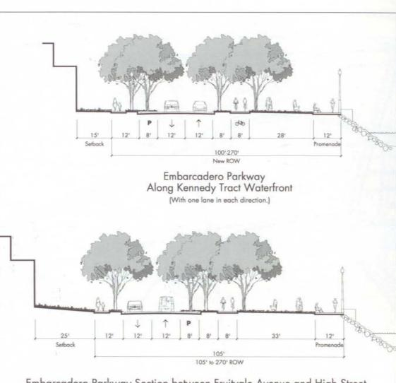
Embarcadero Parkway Section between Fruitvale Avenue and High Street (With one lane in each direction and a single shared turn lane at intersections only.)
