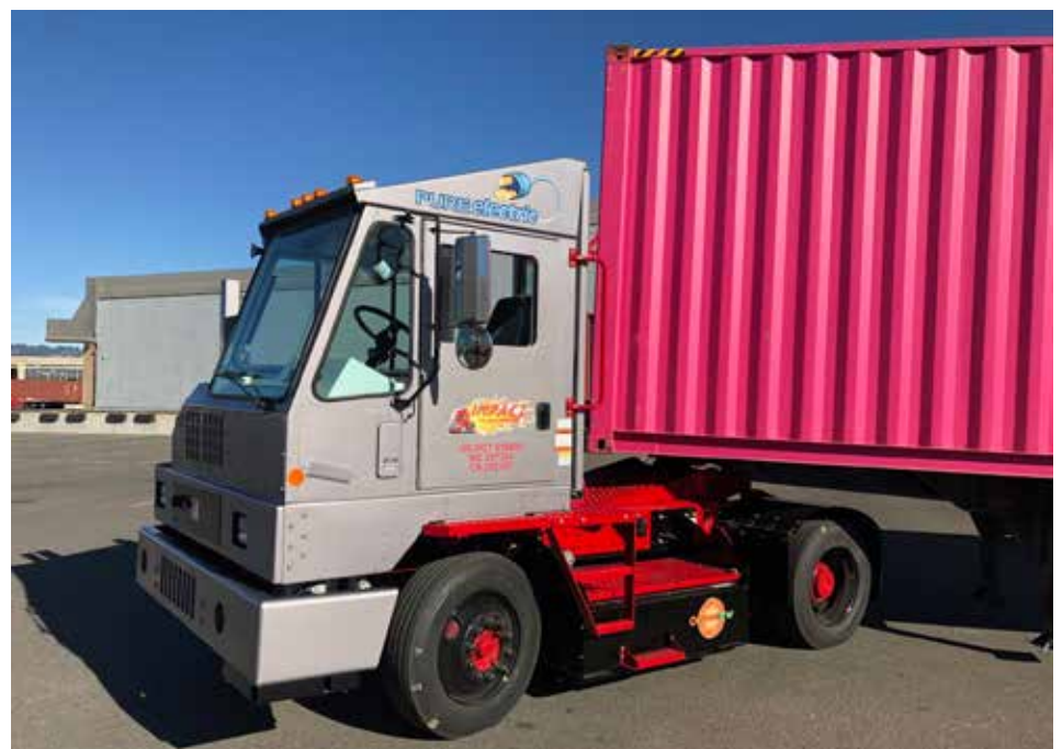
All-electric yard hostler can run for 12 hours on one battery charge.
