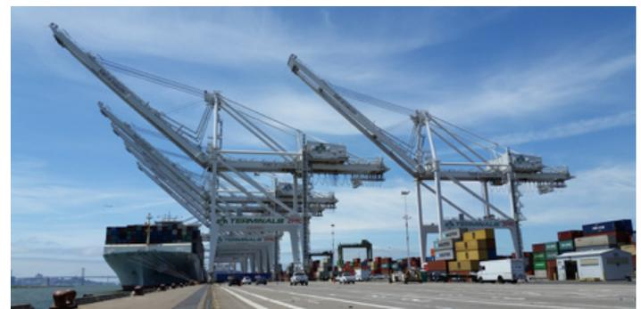
A crane is moved off the line at Oakland International Container Terminal in preparation for raising its height 27 feet
