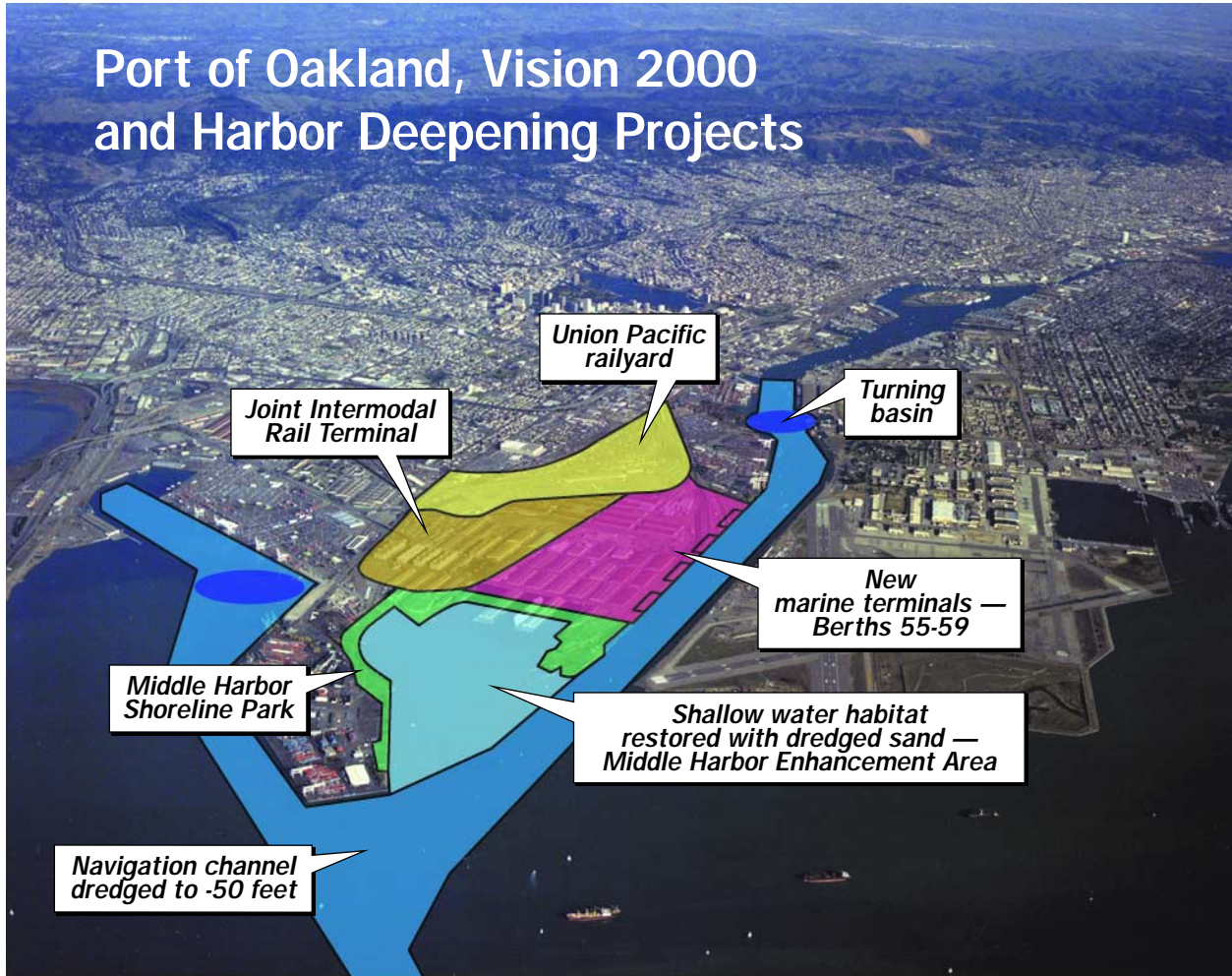
Port of Oakland's Vision 2000 and Harbor Deepening Projects are creating a highly efficient intermodal center for future increases in Pacific trade.
