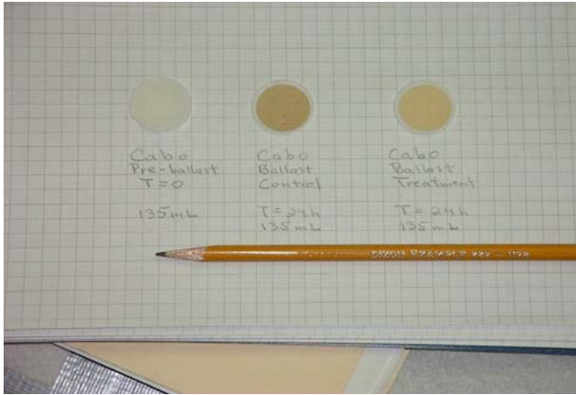
Fig. 8a. Identical 135 mL filtrations onto GF/F glass fiber filters. Left-most filter represents incoming ballasted water from Cabo San Lucas harbor sampled before contact with ballast tanks. Filters on the right were collected directly from the receiving ballast tanks 24 h later.
